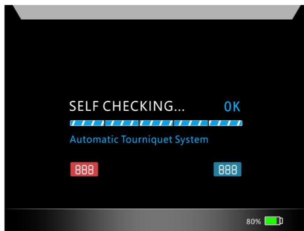
6. After the "self-test" has been successfully completed, the device will automatically display the parameter management screen.
